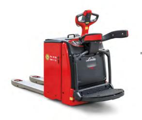
The need to transport goods quickly and precisely over short distances also extends to ATEX zones. To make sure that safety does not suffer, Linde supplies explosion-proof pallet trucks in all necessary payload classes. The trucks are available in a pedestrian design or can be equipped with a driver platform.
