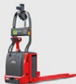
T-MATIC Pallet Truck Capacity: 3.0 t
