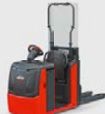
N20-25 C Low-level Order Picker, Man-up Capacity: 2.0 t – 2.5 t Variants: B, HP
