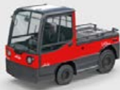
P250 Sit-on Tow Tractor Capacity: 25.0 t Variants: SWB, LWB
