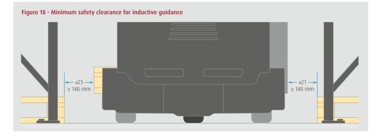
26) Linde: If using a smaller distance, the speed of the truck will be reduced
