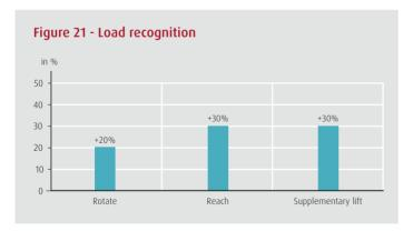
Trucks which are equipped with LSC Weight recognise the total weight of the pallet and its load, and optimise all truck operations accordingly. Light loads can be moved faster than heavy ones. This feature is particularly advantageous in scenarios where loads of differing weights are being handled (see figure 22).
