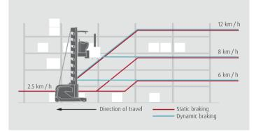
Figure 31 - Individual configuration of restrictions with ASA
